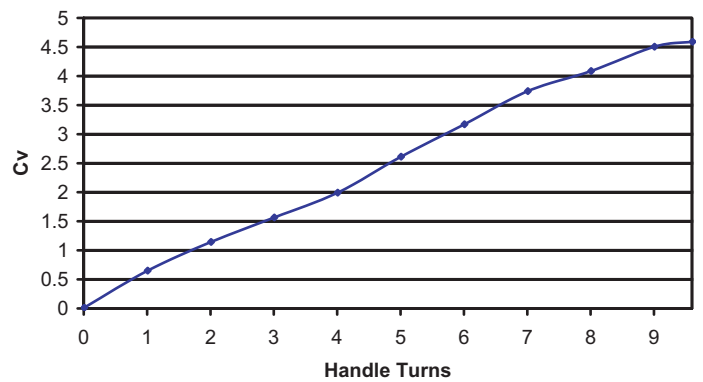
Cv vs Handle Turns for a 8H Throttle Valve with 3/8" Orifice
