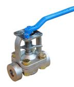
Conval Camseal® ball valves provide zero body, seat, and stem seal leakage. The body/bonnet joint is not subject to pipeline stresses. There is no in-line body bolting to loosen and fatigue. Reliable, accurate ball alignment is achieved due to the robust engagement between the one-piece stem and the ball.
