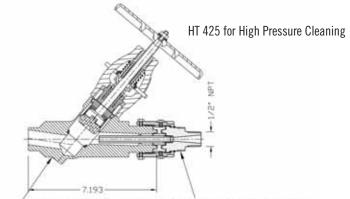
HILTAP 4 PIECE HIGH PRESSURE CLEANING END CAP PARTS HT425-07-HPC-D-3140 CONVAL VALVE WITH INTEGRATED HILTAP MALE HALF
